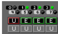
FIGURE 30 Port and LED status color-coded information in the port icon in Switch View
